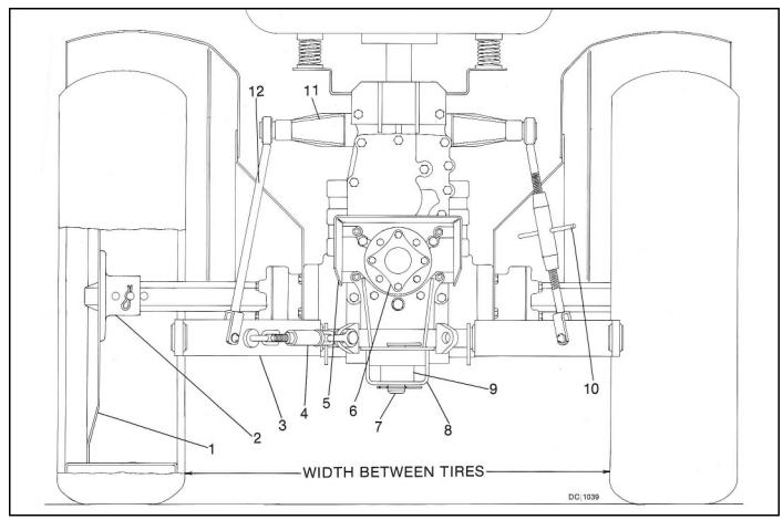
Figure 19. Rear View of Tractor
